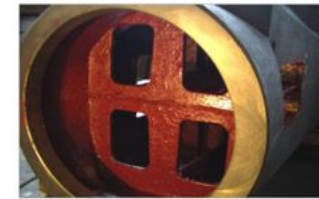
床身箱體結構，增加鋼性 COLUMN:box structure,increase rigidity
