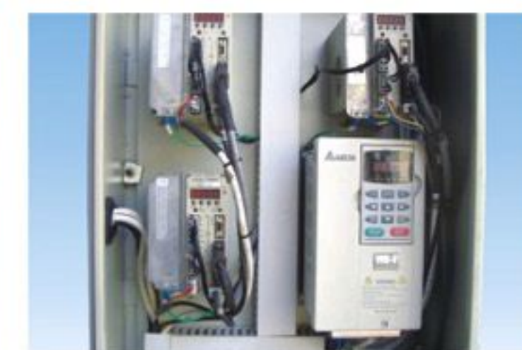
高壓及低壓電器箱分開-減少電波干擾, 避免過熱。High and low voltage Electrical cabinet-Reduce interference & avoid components overheat.
