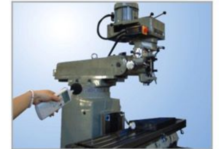
噪音計測試機頭聲音 Detecting noise with noise-meter
