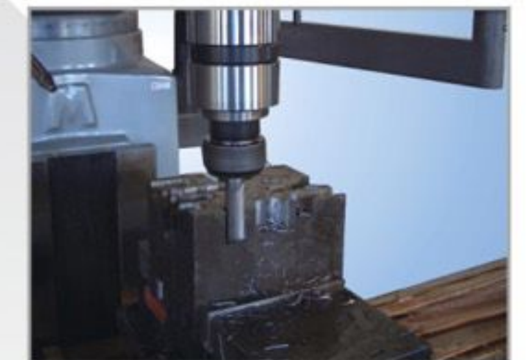
Y軸試切削 Y-axis Test Cut
