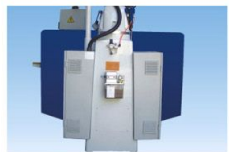
高壓及低壓電器箱分開-減少電波干擾, 避免過熱。High and low voltage Electrical cabinet-Reduce interference & avoid components overheat.
