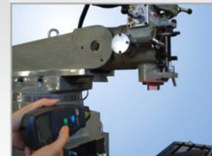
轉速計測試主軸速度 Checking spindle speed with digital tachometer
